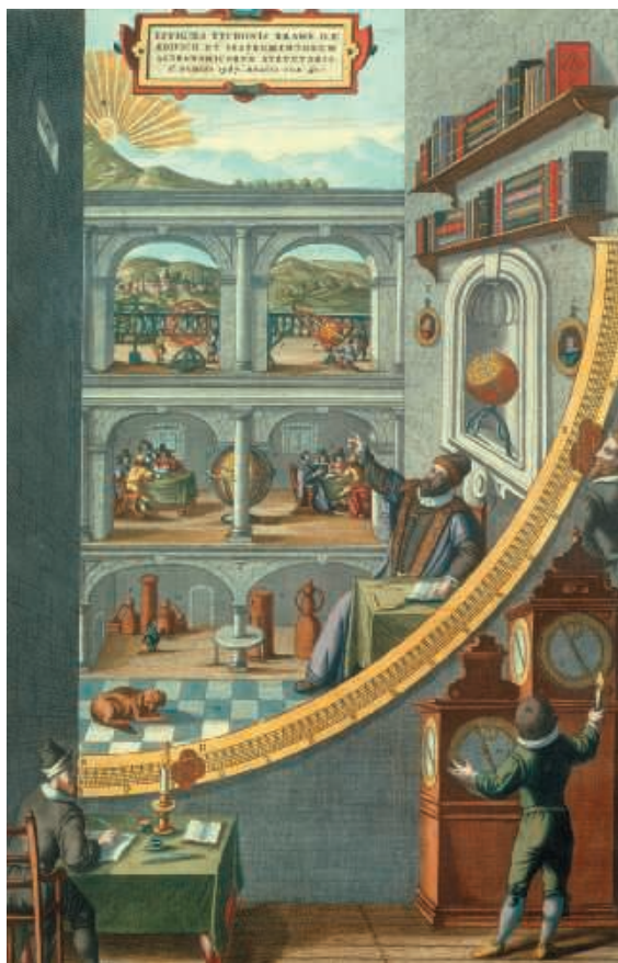
FIGURE 2.7 Tycho Brahe in his naked-eye observatory, which worked much like a giant protractor. He could sit and observe a planet through the rectangular hole in the wall as an assistant used a sliding marker to measure the angle on the protractor.
